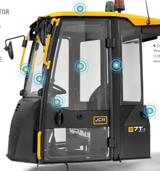
**4.** Detachable for service access and transport. When fitted to a 13,000 lb (6,000 kg) and 15,000 lb (7,000 kg) dumper, overall height remains under 9 feet 10 inches (3 m).
